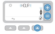
10 Press + or - to adjust the HOUR and press
