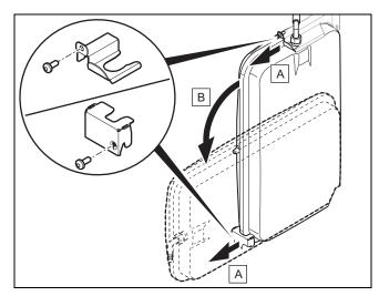
Depending on the components on which you want to work, move the expansion vessel to the maintenance position.
