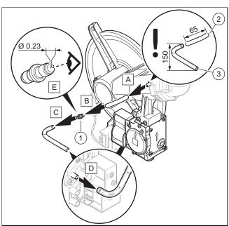
Remove the restrictor for the reference pressure pipe
