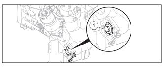
3. Regulate the pressure using the adjusting screw (1).
