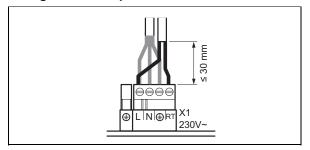
► Connect the control to the *L* main plug and to the *RT* plug.
