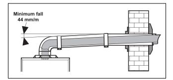
Standard flue terminal kits have an in-built fall back to the boiler to drain the condensate. These can be fitted level between the appliance and the termination position. All other extended flues must have a fall of at least 44 mm/m.
