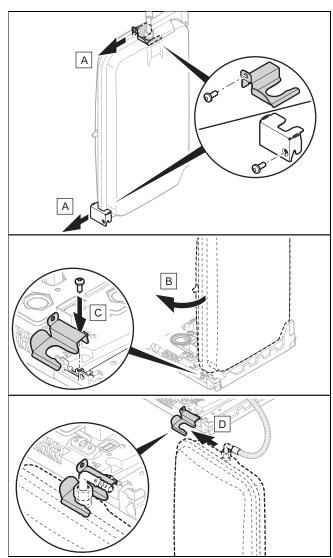
Depending on the components on which you want to work, move the expansion vessel to the maintenance position.
