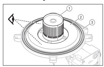
1. Check the surface of the burner (1) for damage.
