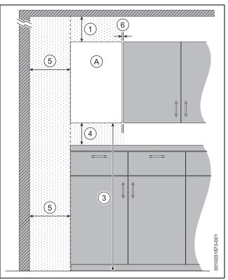
Fig. 12 Reduced front maintenance clearances - Front view
