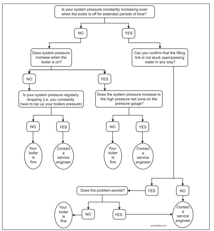
Fig. 13 Gassing flow chart
