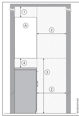
Fig. 11 Reduced front maintenance clearances - Side view
