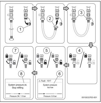
Fig. 8 External filling loop
