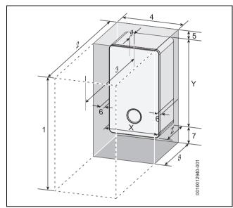
Fig. 10 Appliance minimum clearances
